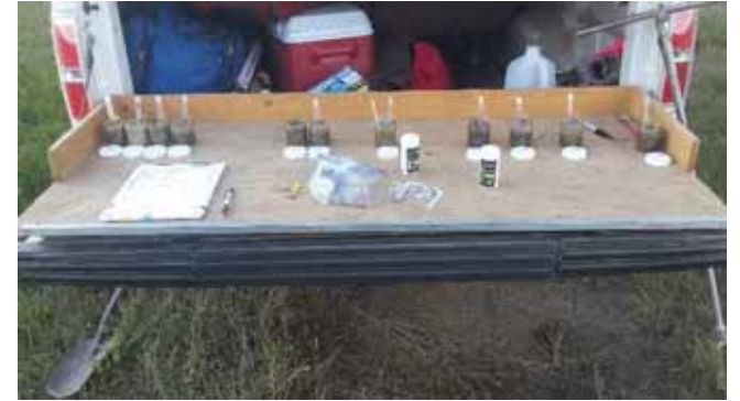
Chloride testing in the field.
