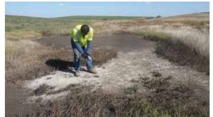
Field screening soil with EC meter.
