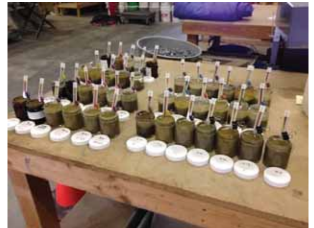
Chloride test from samples collected.
