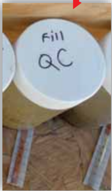
Sampling of the backfill prior to being placed in excavated area for quality control.
