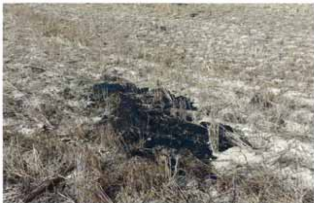
Petroleum hydrocarbons at surface from historical piping that leaked.
