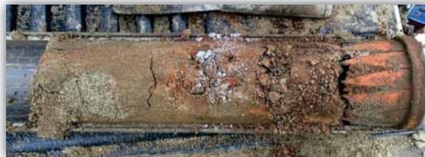
Split-spoon soil sampling – scoria, shale cuttings, and petroleum hydrocarbons.
