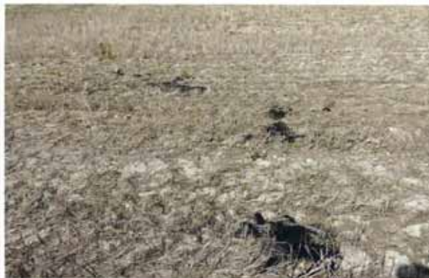
Petroleum hydrocarbons at surface from historical piping that leaked.
