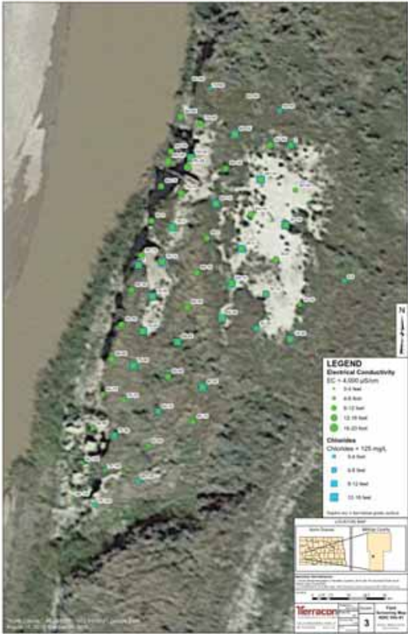
Field screening results (after excavation) up to 20 feet bgs.
